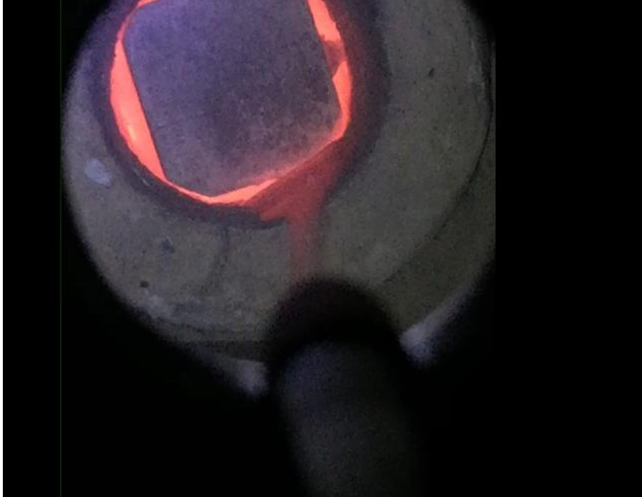
Figure 4B: View of the unit stopped and opened during reclaiming process showing waste sand at the entrance and reclaimed sand exiting the unit.
