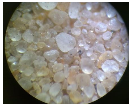
Reclaimed sand after microwave processing
